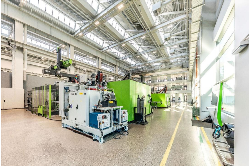
The ENGEL clearmelt-Competence-Center demonstrates how customers can efficiently achieve high-quality, scratch-resistant surfaces through a fully integrated PUR solution and centralised project management. Shown here: a test setup with a duo 1800 two-platen injection moulding machine and PUR dosing system.
